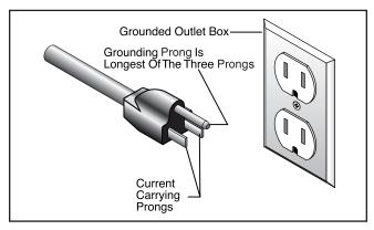
**Figure 1.** Typical type 5-15 plug & receptacle.
